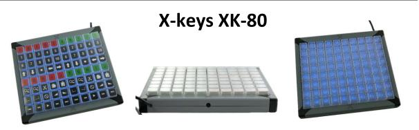
The XK-80 offers an 8 x 10 grid of programmable keys to trigger macros, shortcuts, and applications, select tools or open files or directories. Key blockers can knock out unused keys and delineate groups to instantly create a custom control panel.
